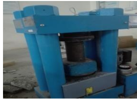
3.2.1 Compressive strength Test
